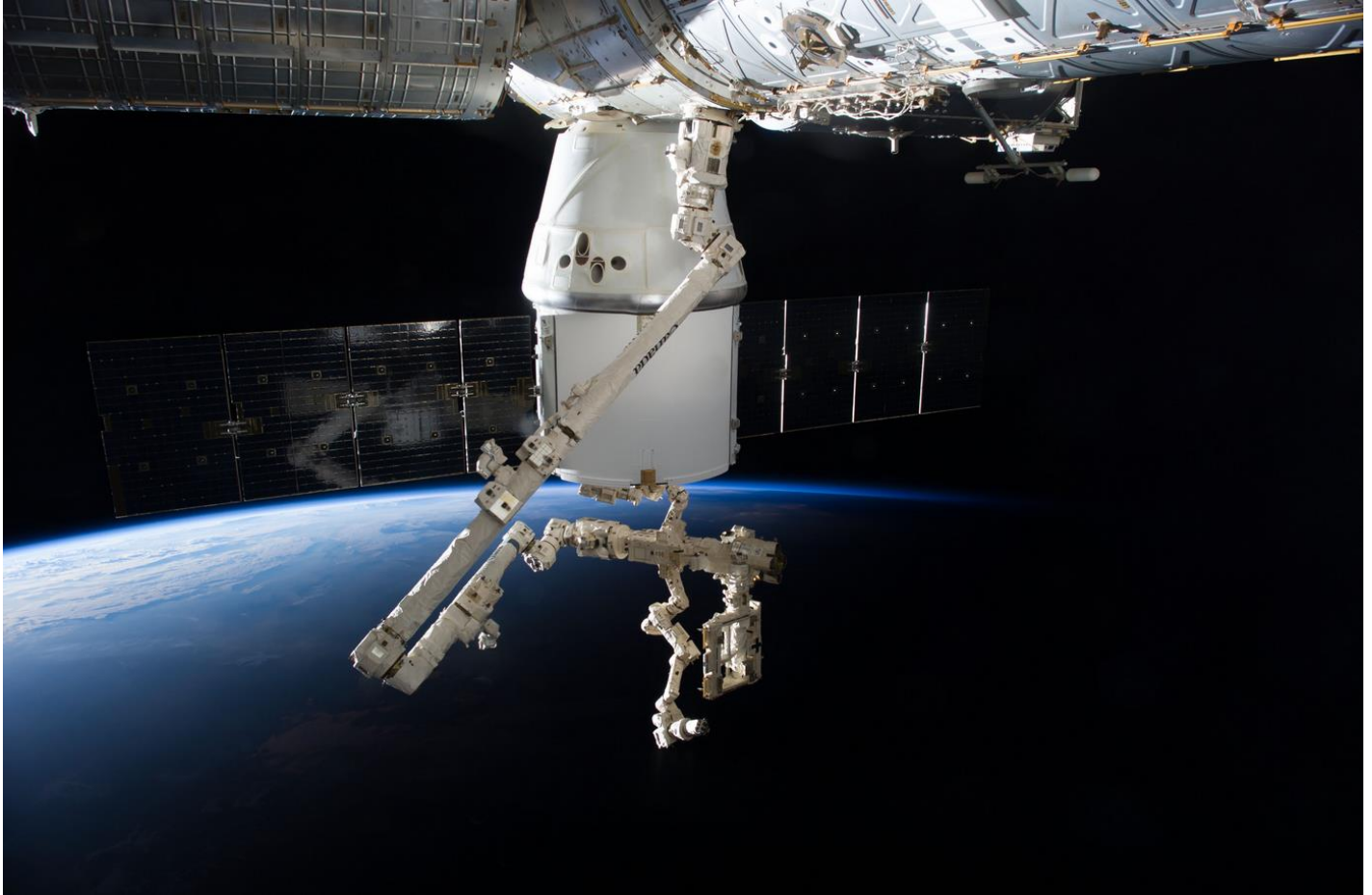
Figure 34: SSRMS on the ISS Reaching into the Dragon External Cargo Bay 84
