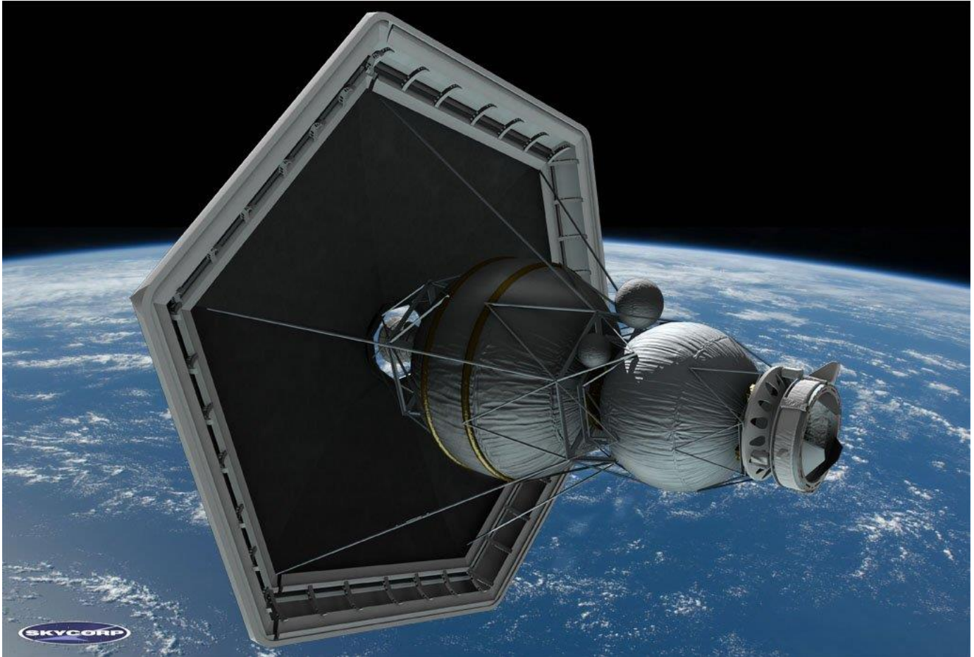
Figure 66: Reusable Lunar Orbital Transfer Vehicle Concept Using Aerocapture 148
