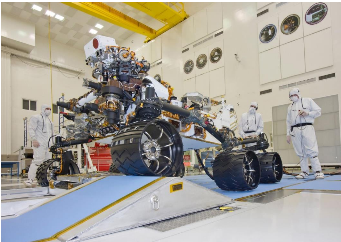
Figure 55: MSL Articulated Wheels and Traction Treads 126
